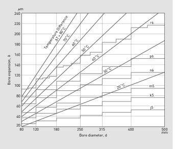
Therefore, 70% to 90% of the interference appears as reduction in clearance. (Smaller reduction in clearance is adopted for bearings of diameter series 4.) Moreover, the difference in operating temperature between inner and outer rings ranges from 5°C to 10°C. However, this temperature difference will exceed that range if the inner ring's temperature rises or the outer ring is cooled. Reduction in clearance due to temperature difference between inner and outer rings:
