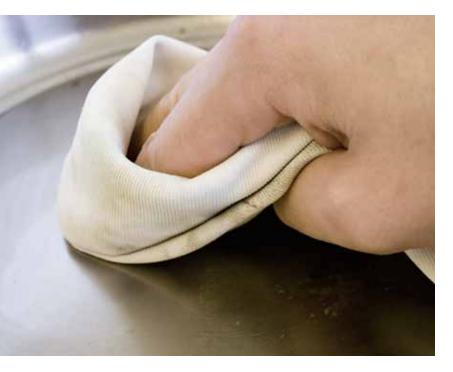
Nevertheless, removing the anti-corrosion agent is recommended for small bearings used in high-speed operations or for bearings that will use low-viscosity or mist lubrication.
